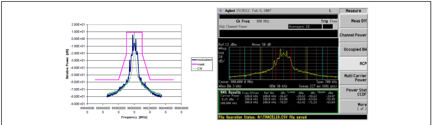
Figure 36: Indy R1000 Reader Chip Transmit Modulation and Mask for SSB, Tari=25 μsec, X=1
